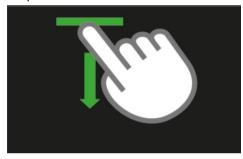
Open the Infotainment control centre by holding down the bar at the top of the screen and pulling it down.
