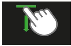
Open the Infotainment control centre by holding down the bar at the top of the screen and pulling it down.
